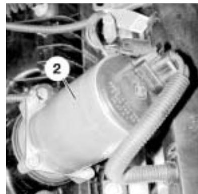
**Valvetronic Sensors:** Each eccentric shaft is monitored by a magneto-resistive position sensor. The N62 engine has two sensor assemblies, one for each eccentric shaft. These sensors are very durable for the environment (inside the cylinder head) and cope well with vibrations and high temperatures. The sensor assembly consists of:
