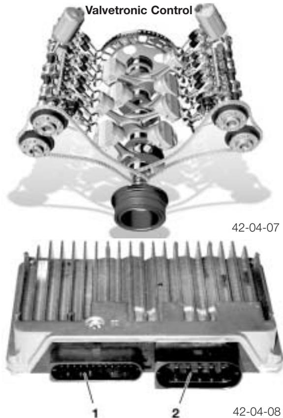
**Valvetronic Motors:** Two DC motors (2) are fitted to adjust the two eccentric shafts. They are operated at a frequency of 16 kHz in order to make exact adjustments. In order to position the motors exactly, the polarity is briefly reversed once the target position has been reached (as identified by the ECM). This generates braking torque which immediately stops the motors.
