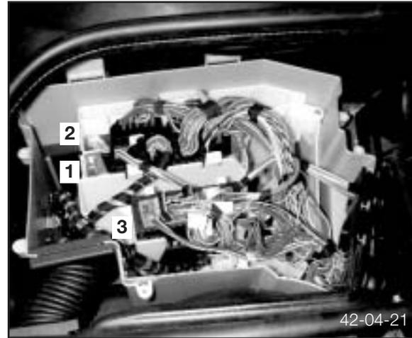
The ECM controls an electric cooling fan in the base of the electronic box to draw in cool air from the passenger compartment.
