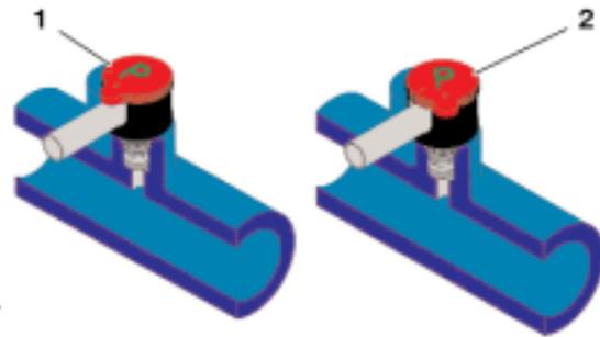
*Prior to reconnection, the cap must be reset to the locked operating position (1) and should be plugged into the connection only in this position.*
