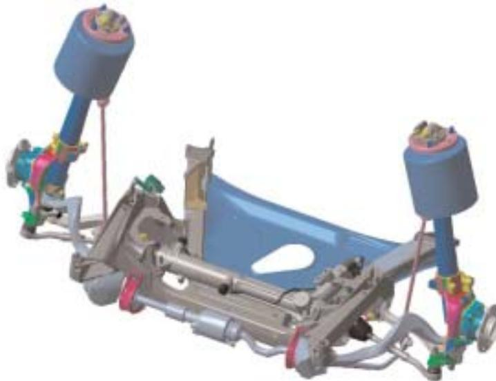
**Front Axle Carrier:** The materials used in the front axle carrier offer high tensile strength to support extreme loads. The front axle carrier is also manufactured from aluminum. It consists of cast alloy preformed sections which are welded into the extruded sections.
