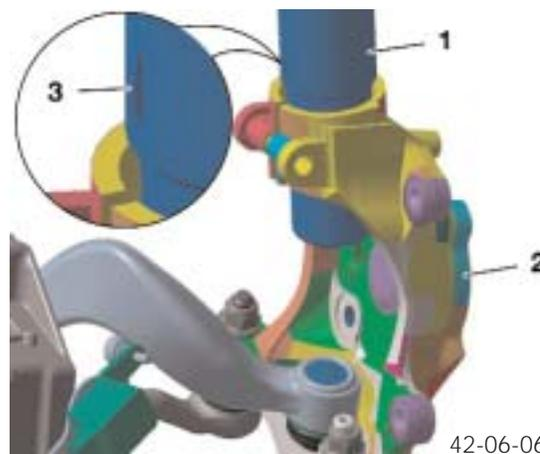
Spring Strut, Hub Carrier, and Wheel Bearing
