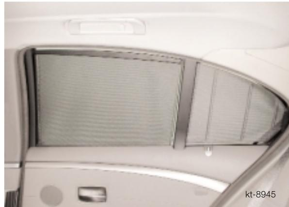
When the window is open and a command to raise the side-window roller blind is sent, the side-window roller blind starts up briefly and reverses. This indicates that an invalid operation has been attempted. The roller sun blind cannot be raised until the customer closes the window. It is always possible to operate the quarter roller blind, irrespective of the side window position.
