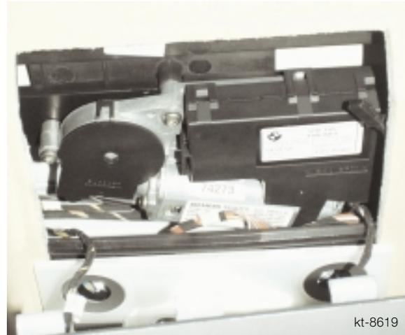
The DC motor is controlled with a PWM signal to provide a smooth-rundown feature similar to the window operation.
