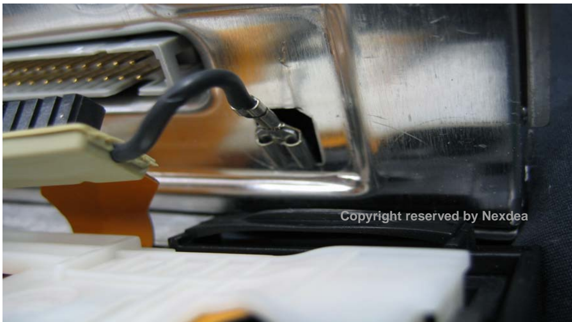
Picture 15. Remove GND connector next to film-cable connector
