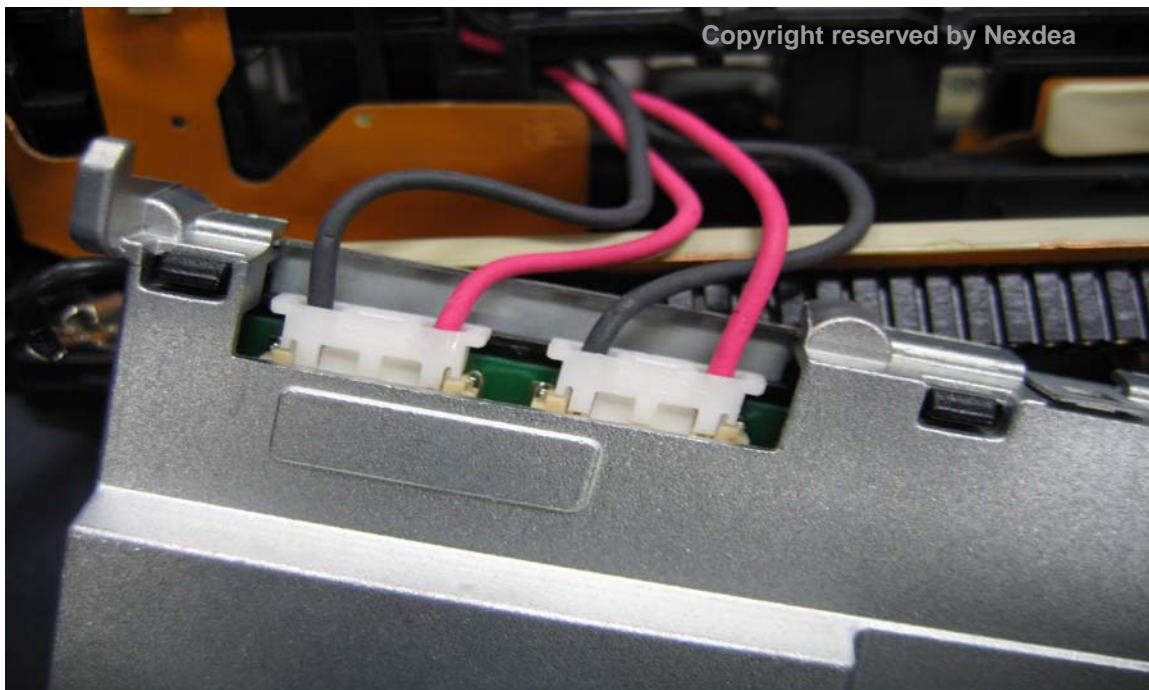
Picture 43. Assemble inverter power cable
