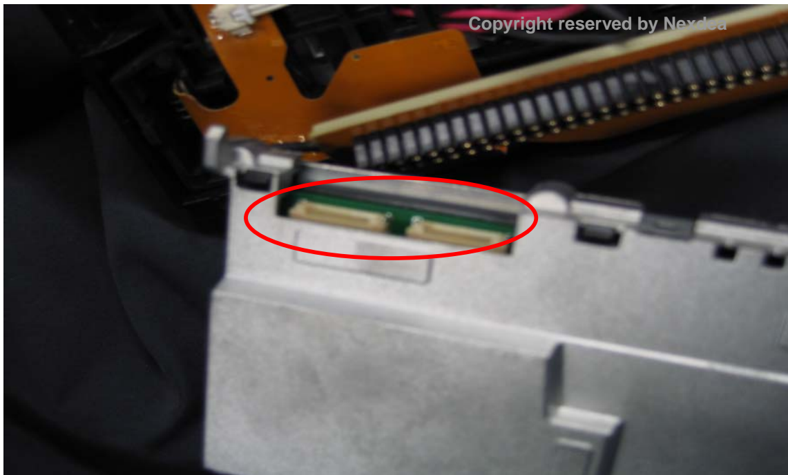
Picture 29. Remove inverter module – 10 : remove power cable connector
