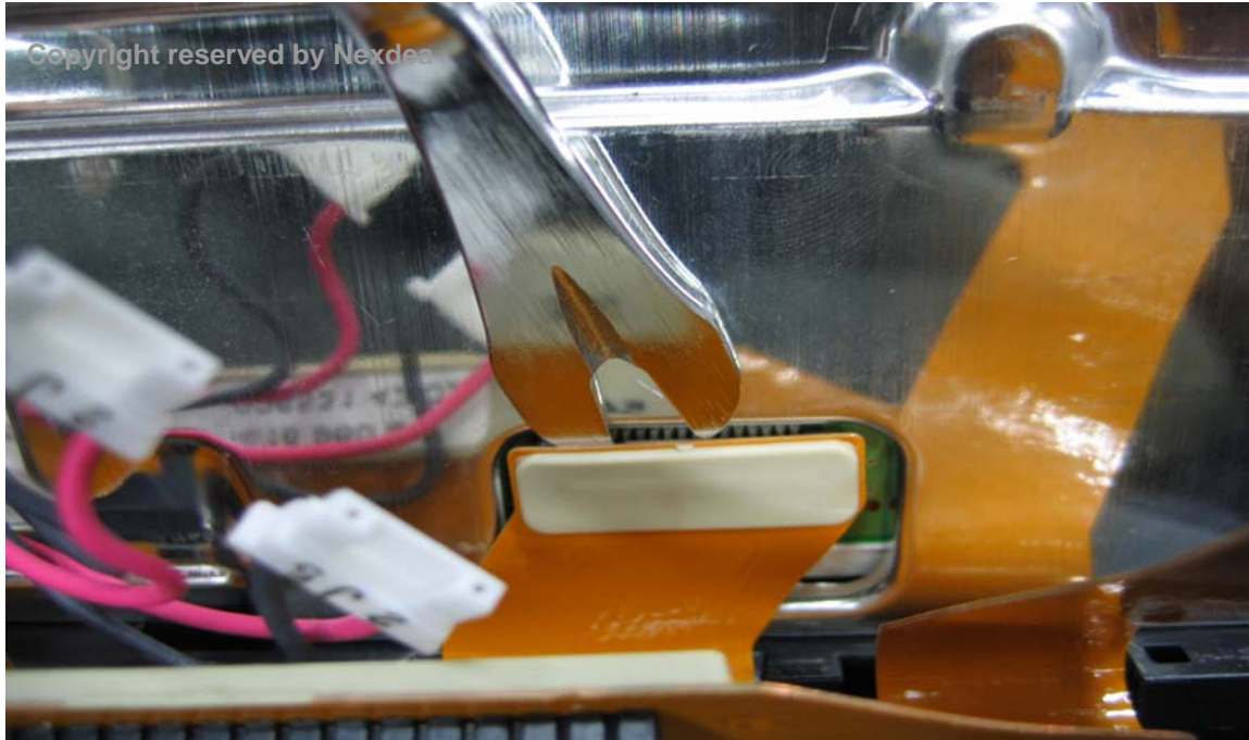
Picture 32. Remove LVDS film-cable from LCD panel - 1
