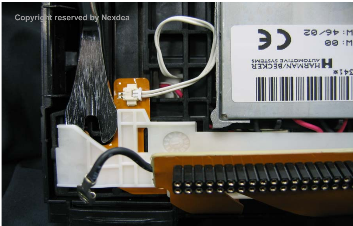
Picture 20. Remove backlight inverter module – 1 : remove white plastic cover
