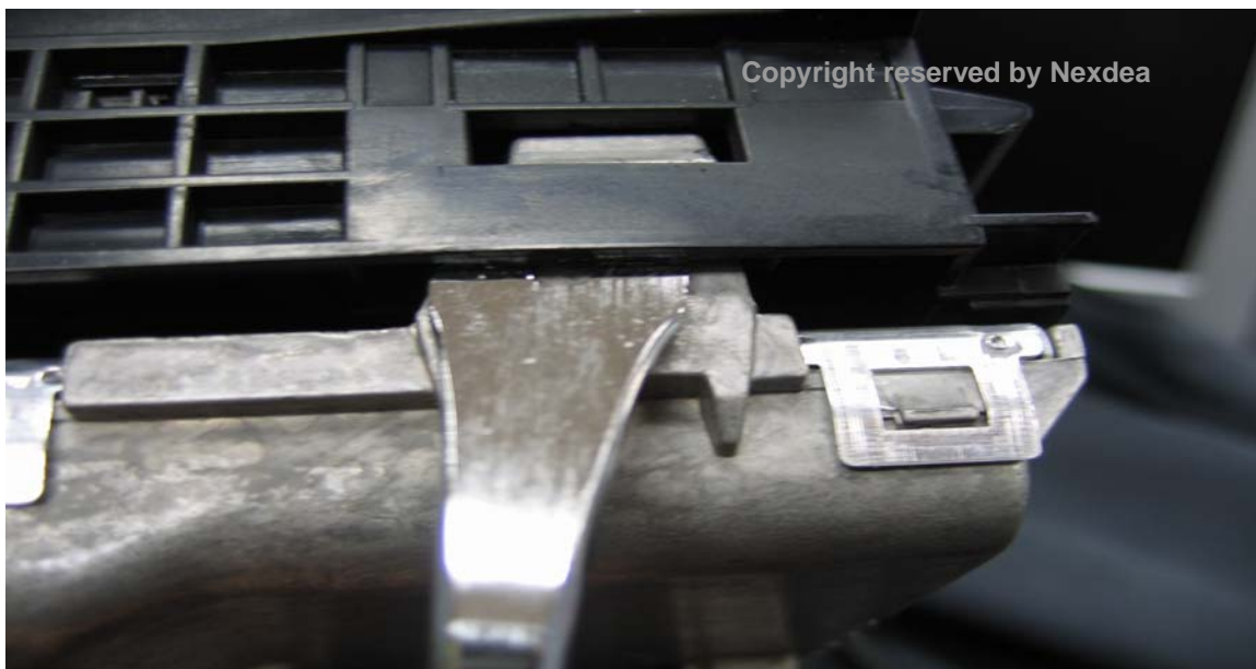
Picture 7. Remove plastic cover with proper tool - 1
