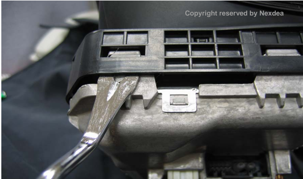
Picture 8. Remove plastic cover with proper tool - 2
