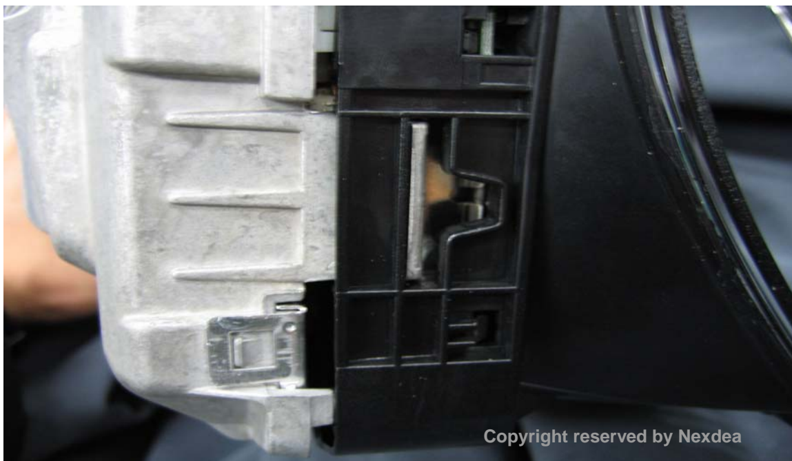
Picture 53. Assemble metal cover and plastic cover - 1
