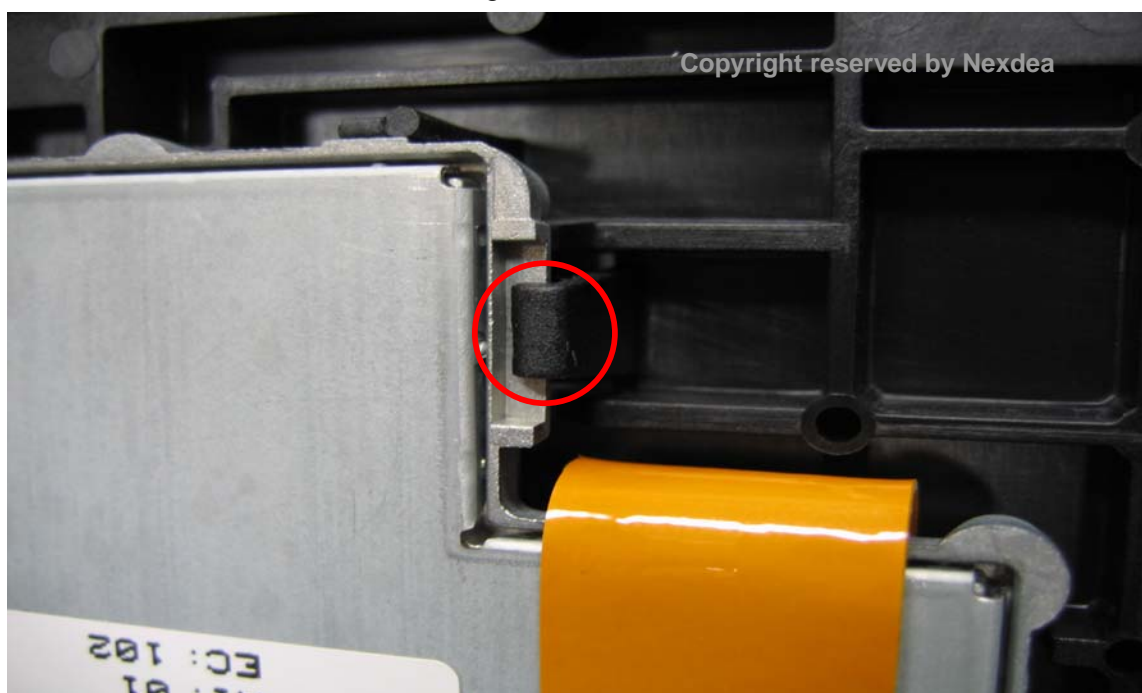
Picture 47. Assemble locker holding inverter module
