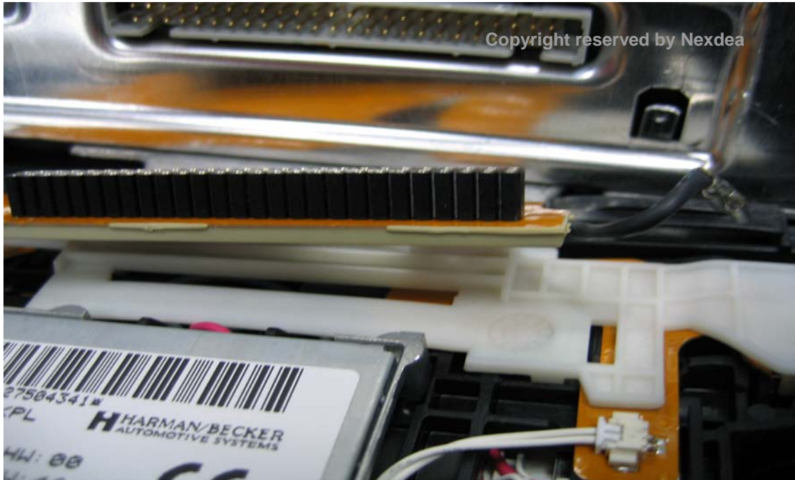
Picture 17. Status after disassemble LVDS connector and GND connector
