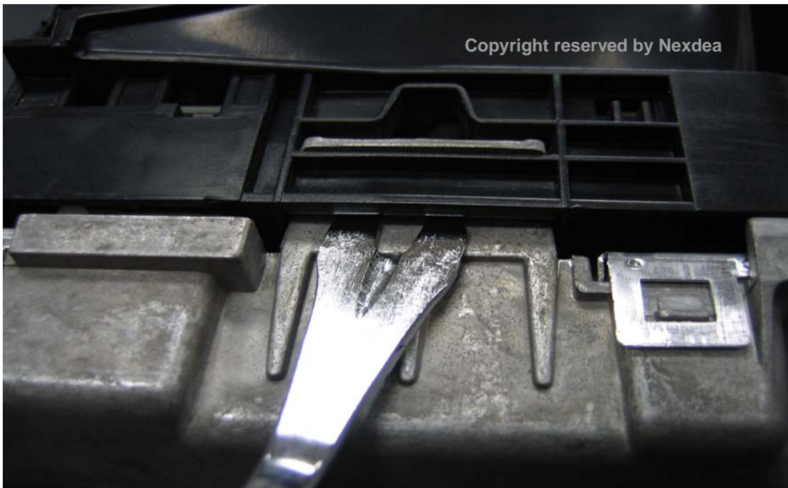
Picture 12. Remove plastic cover with proper tool on other side - 2
