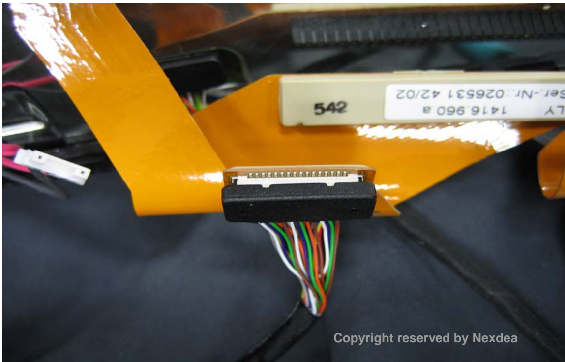
Picture 37. Connect supplied LVDS cable with LVDS jack on film-cable - 2
