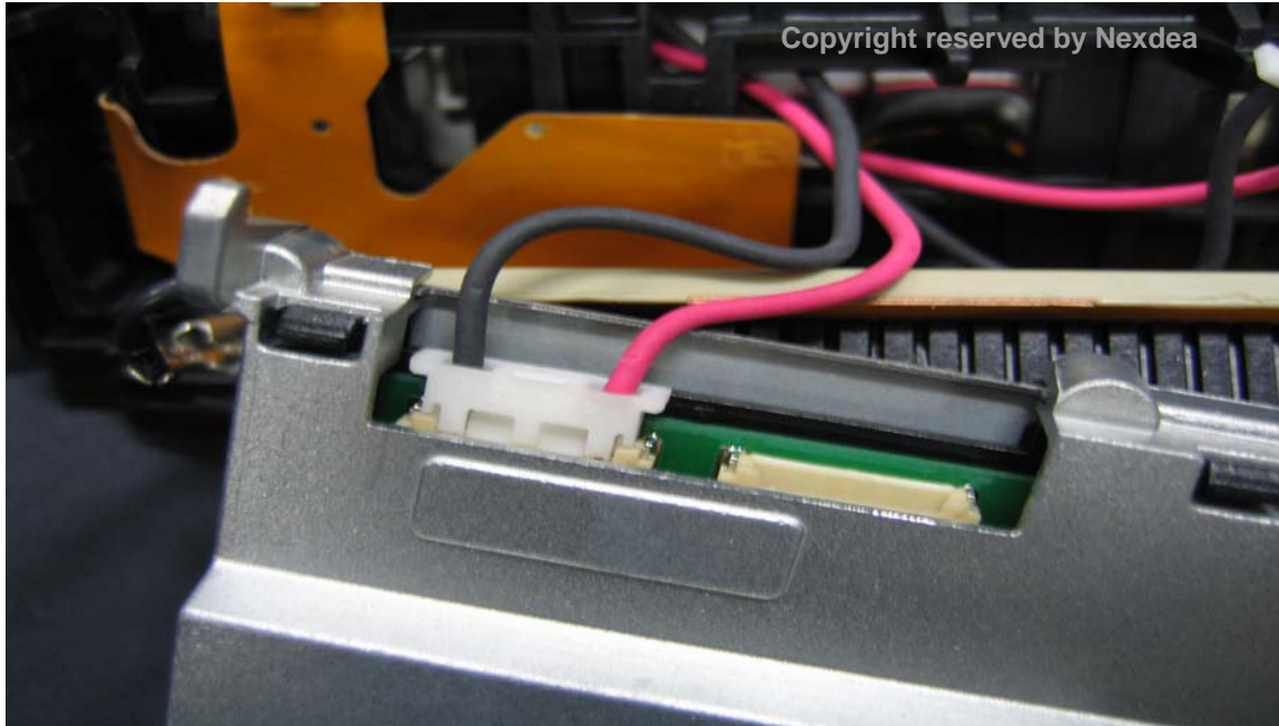
Picture 42. Assemble inverter power cable
