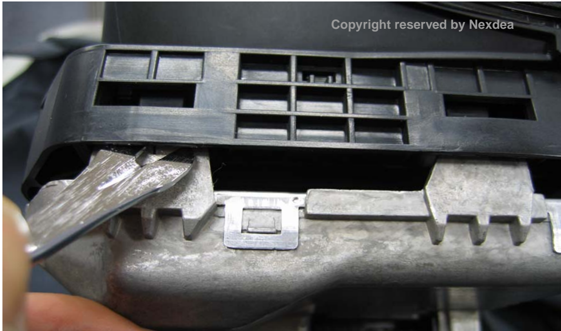
Picture 9. Remove plastic cover with proper tool - 3
