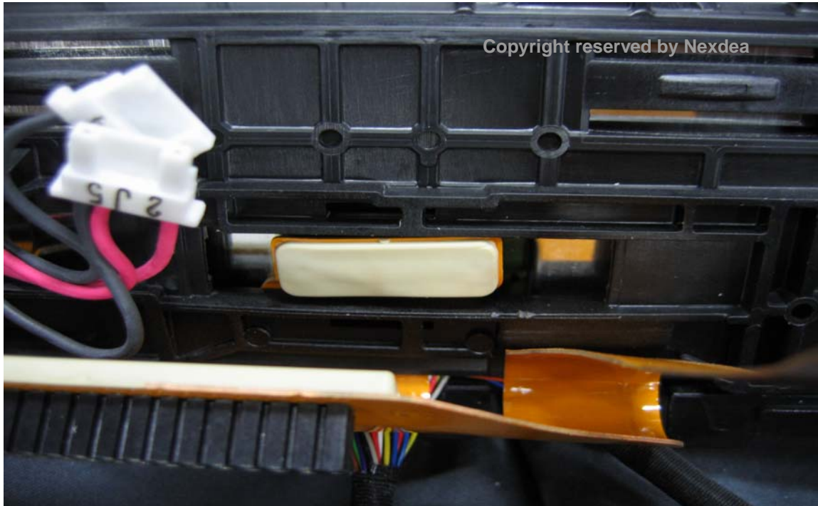
Picture 38. Break small plastic bar to ease tension on LVDS jack (not mandatory)
