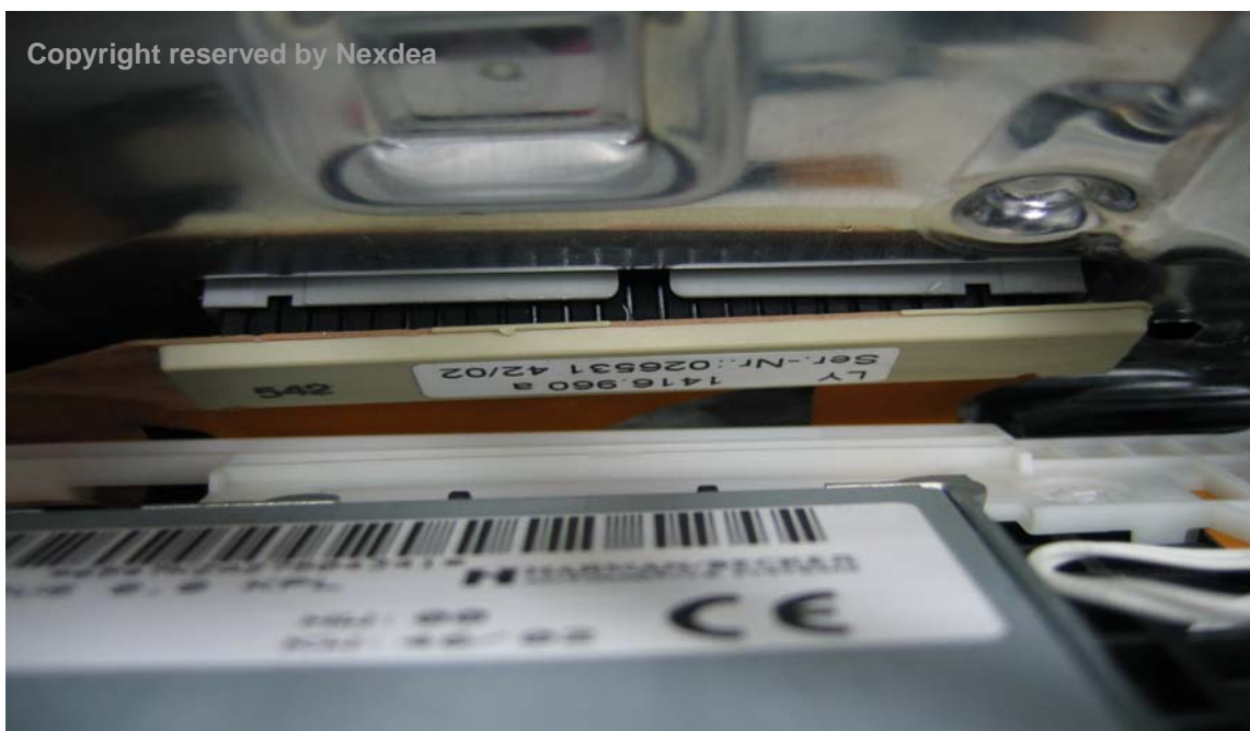
Picture 51. Connect LVDS connector - 1
