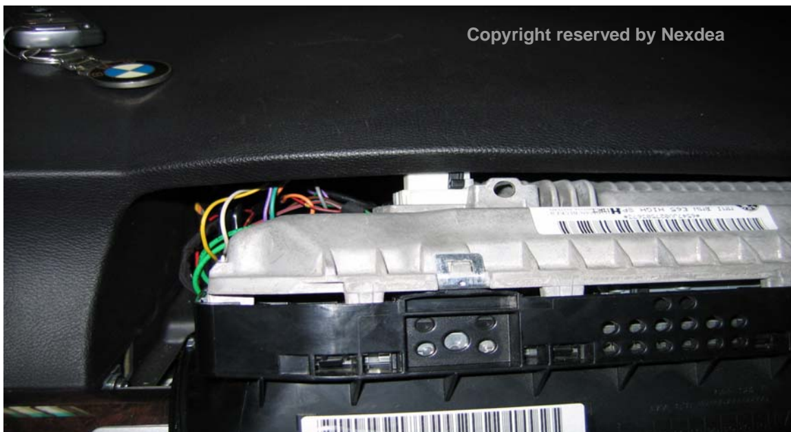
Picture4. Pull out monitor module - 2
