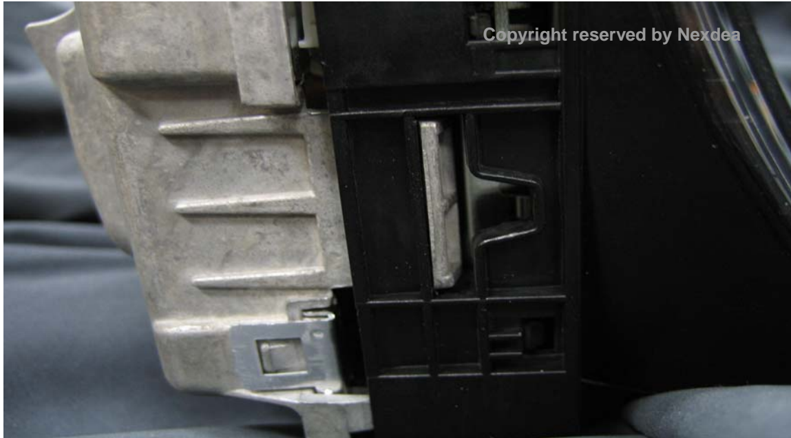
Picture 54. Assemble metal cover and plastic cover - 2
