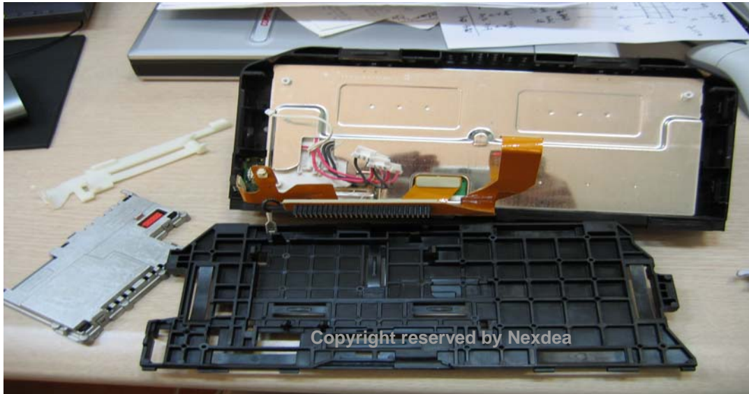
Status after finishing removal of backlight module and LCD cover
