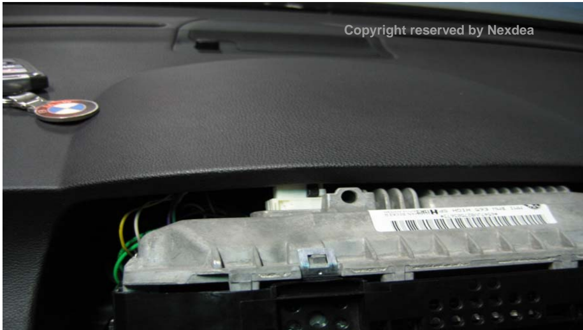
Picture 3. Pull out monitor module - 1
