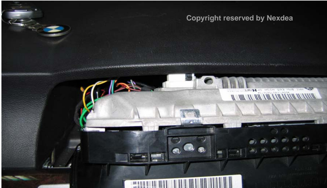
Picture4. Pull out monitor module - 3
