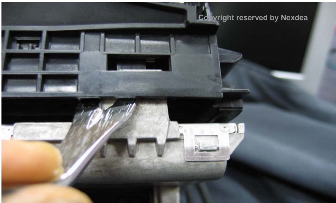
Picture 10. Remove plastic cover with proper tool - 4
