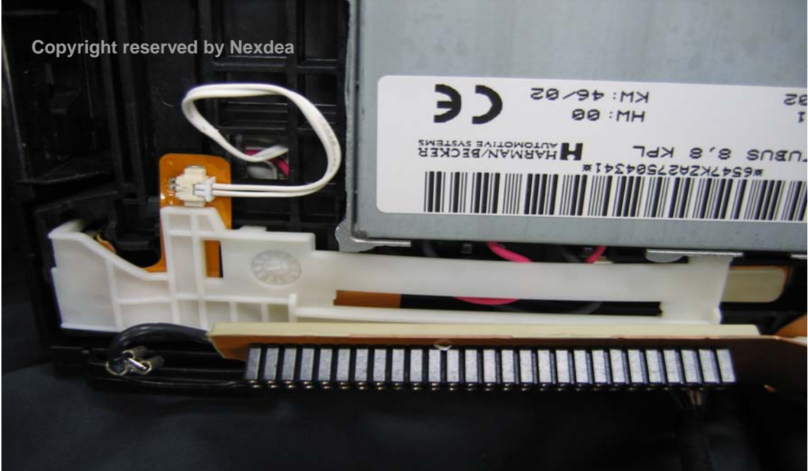
Picture 48. Assemble white plastic cover holding film-cable and LVDS jack
