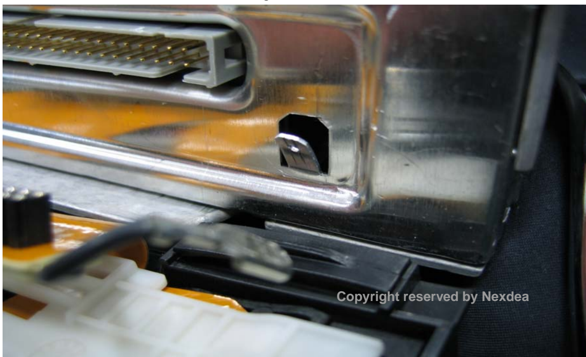
Picture 16. Status after disassembling GND connector
