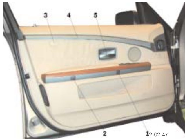
Front Door Mounting Screws
