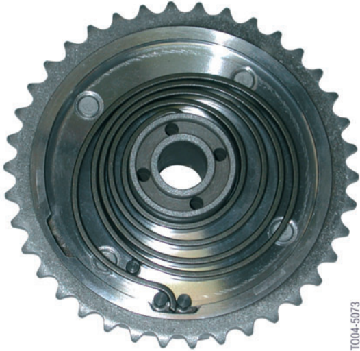
26 - Rear view of VANOS unit with cover removed
