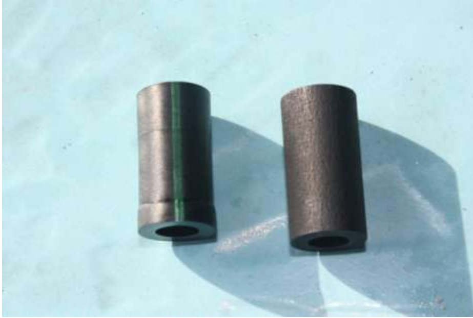
Figure 17 Old Sleeve Left New Right
