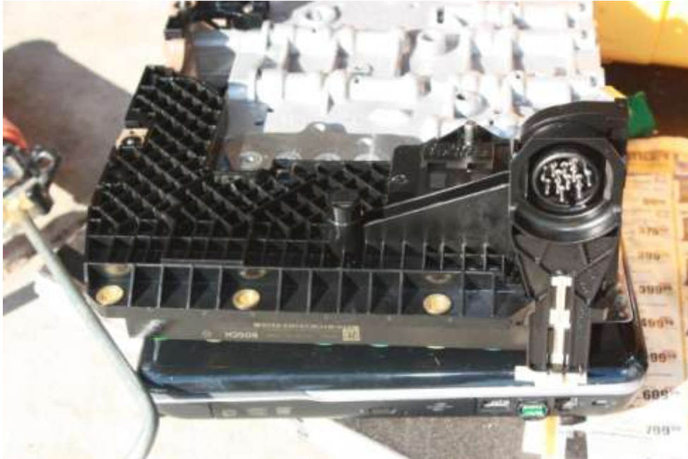
Figure 14 All Clean and back Together
