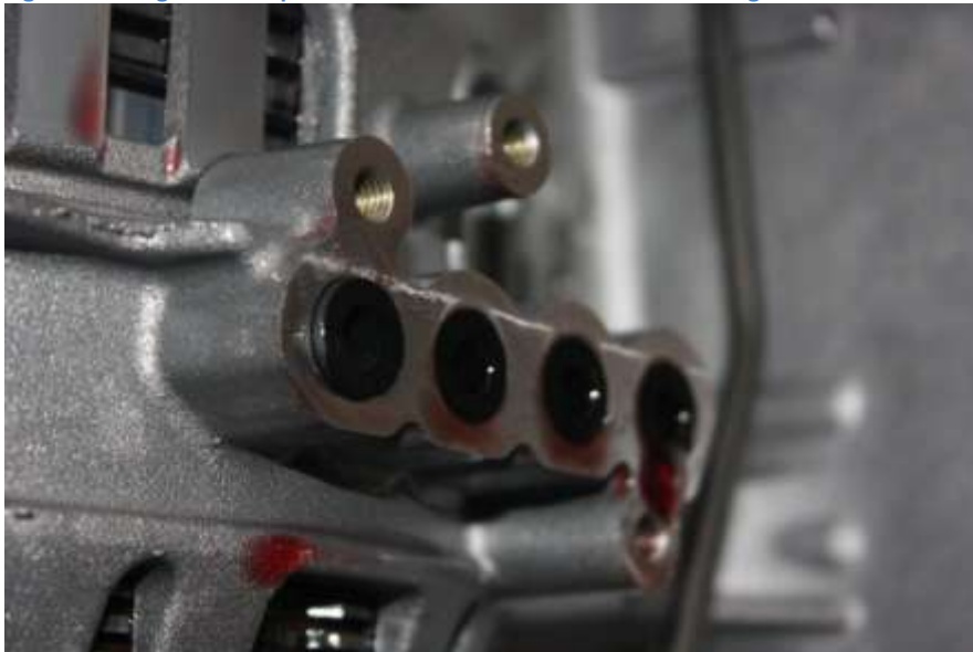
Figure 16 The 4 Sealing Sleeves Replace while its easy
