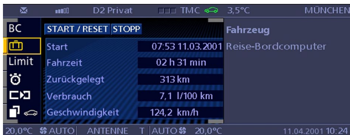
Fig. 18: Menu of the travel computer in the Control Display with display of starting time, driving time, distance travelled, average fuel consumption and average speed.
