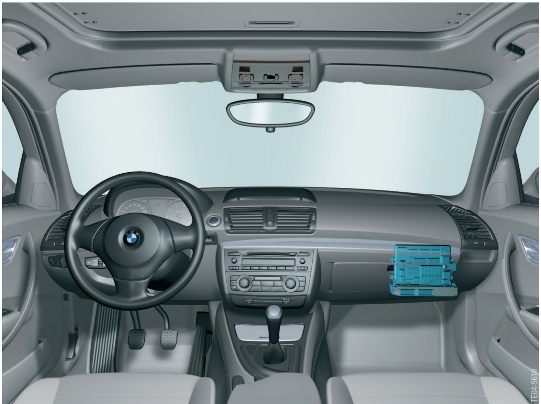
10 - Installation location, junction box
